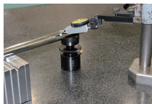
Measuring round bar by use of V-groove attachment
