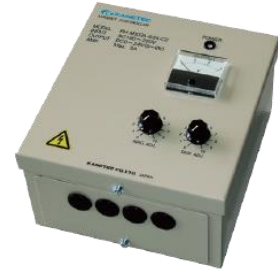
RH-M303A-6/24-C2 [Type housed in case] The base construction is the type installed inside panel. This is placed in a dedicated case to enable installation on the side face of a machine. This type is equipped with a power indicator lamp, voltmeter, magnetic force adjust variable resistor and demagnetizing variable resistor.
