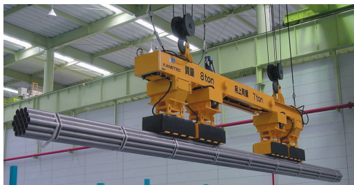
(Lifting bundled pipes)
