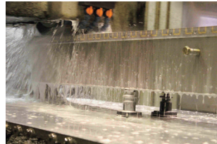
Supporting the hollow portion during grinding
